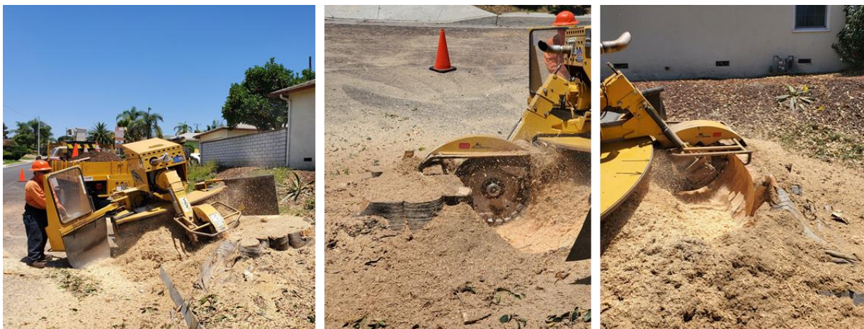
Stump grinding a residential tree ( Ficus elastica ). Photo credit: Dane Jensen, West Coast Arborists, Inc.
