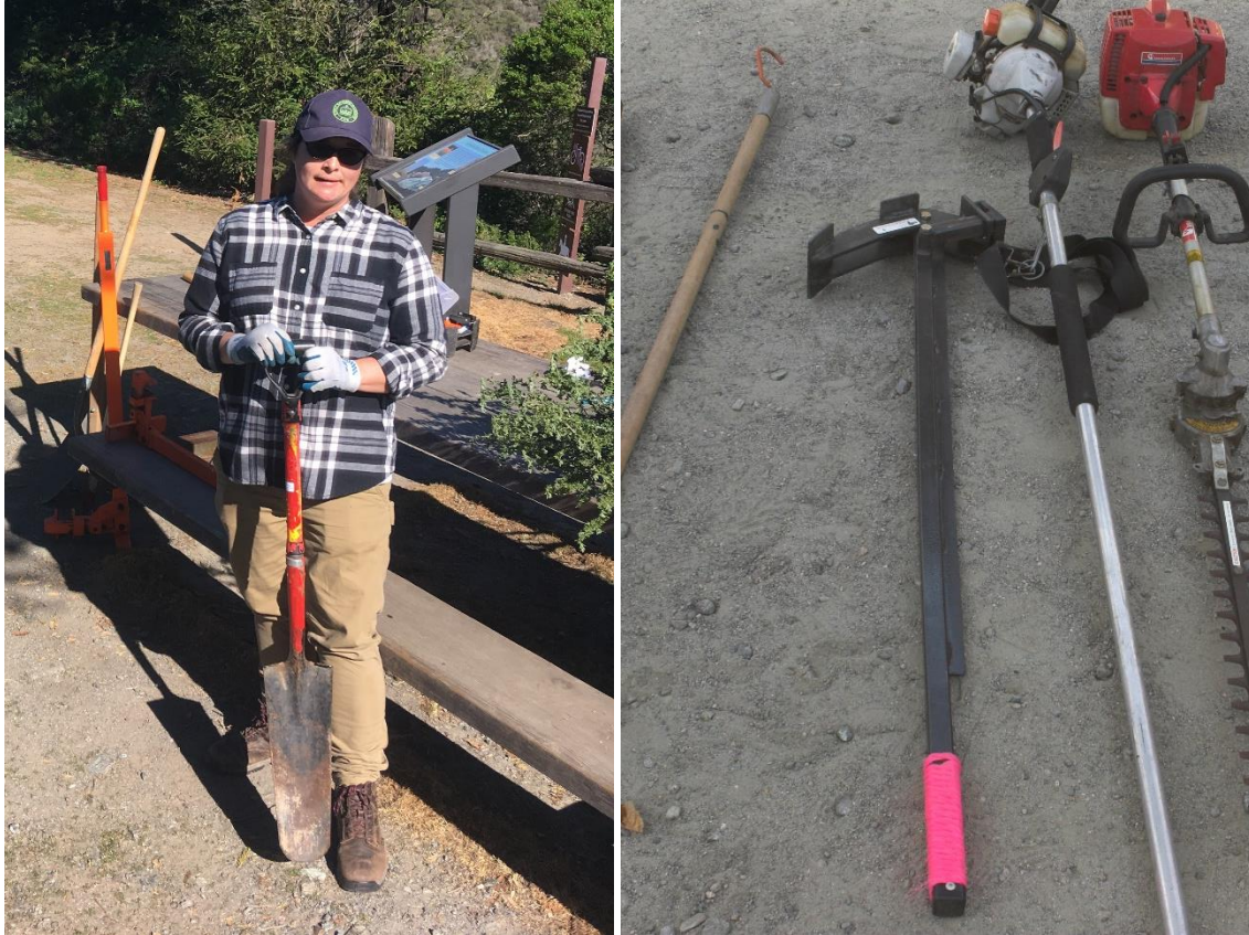
Manual removal tools for shrubs. Left: Sharpshooter shovel (Photo credit: Dana Morawitz). Right: Weed wrench Photo credit: Cal-IPC.
