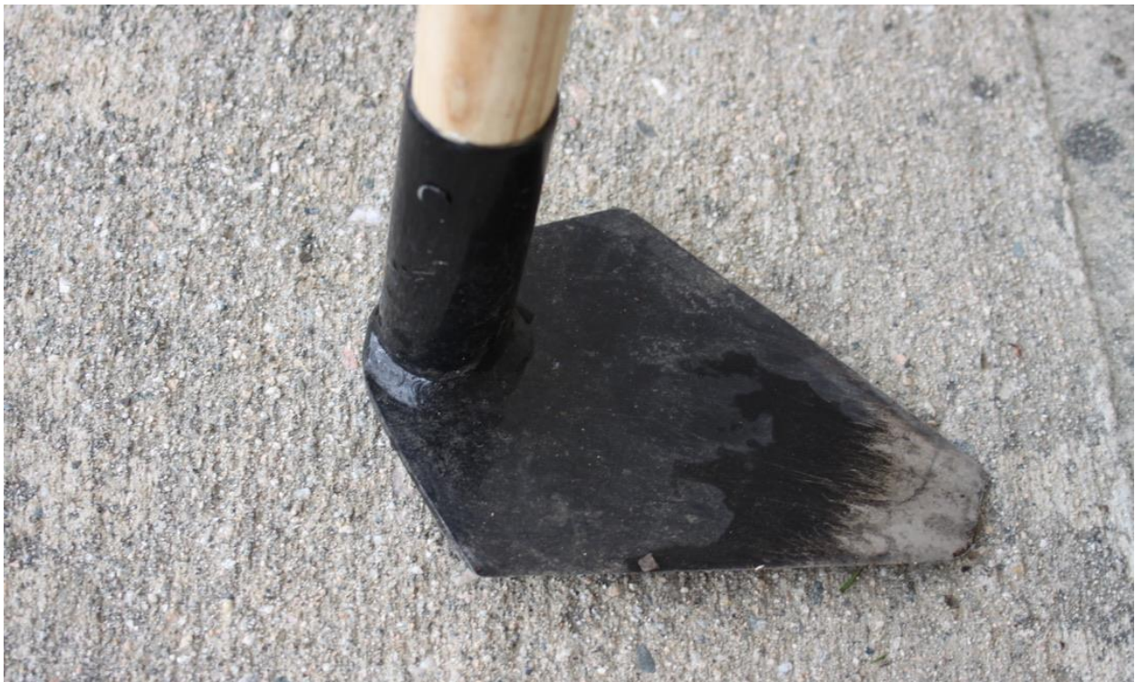
A triangle-shaped grub hoe, with a blade tapering from 5 in. wide at the widest to 1.25 in. wide at the tip. Photo: Christopher McDonald
