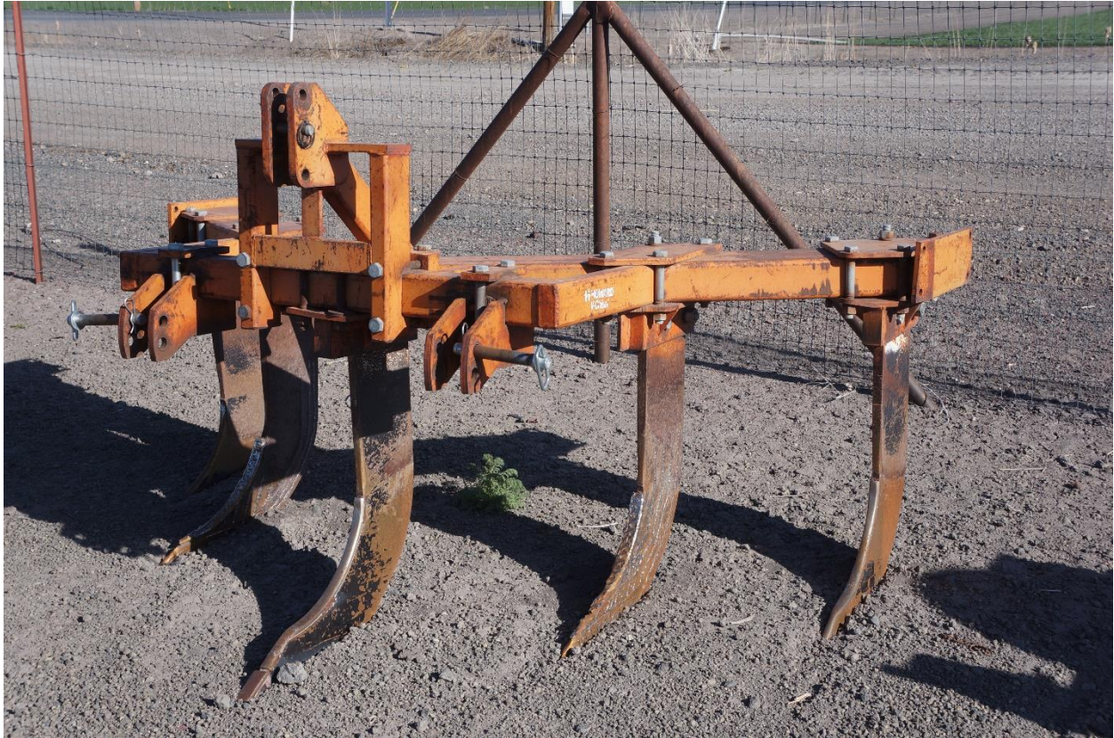
Ripper attachment. Photo credit: Kevin Nicholson.
