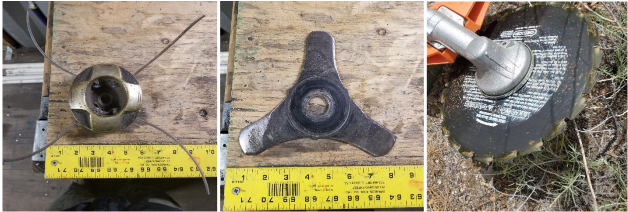
Three weed trimmer head attachments for tougher vegetation. Left: Heavy-duty fixed-line trimmer head. Center: Tri-bladed brush-cutter blade. Right: Circular brush-cutter blade (for woody material). Photo credits: Shawn Thorin (Left, Center); Tom Getts (Right).
