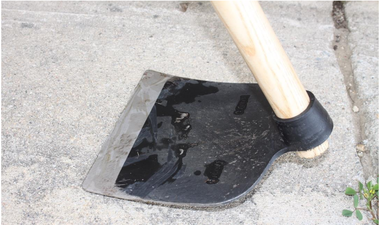
This 8"-wide grub hoe, also called a grape hoe, has a curved blade. Photo credit: Christopher McDonald.
