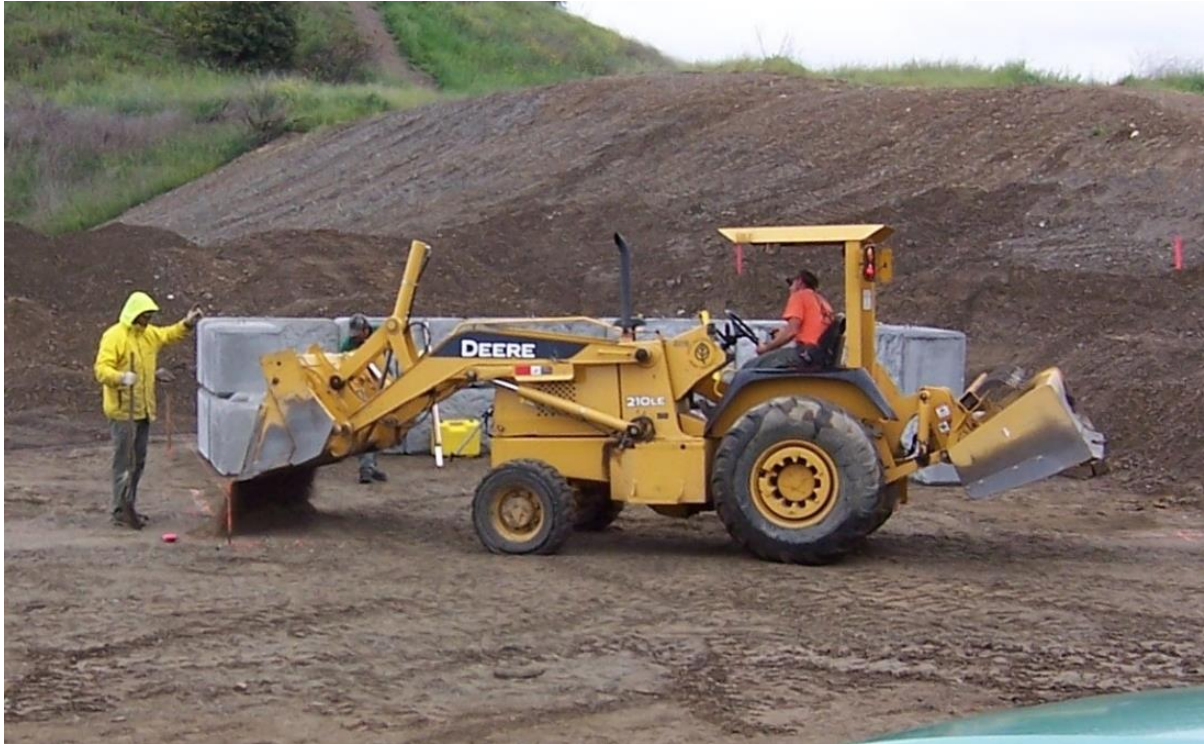
Skip loader with articulating bucket on front and box scraper on back.. Photo credit: Rodney Smith, East Bay Regional Parks District.
