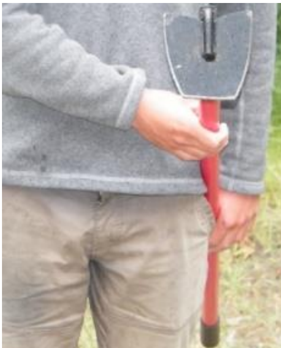
Two modified tools for removing artichoke thistle rosettes. Left: Triangle hoe with tip cut off and edge sharpened (Photo credit: Sandy DeSimone). Right: Shovel bent, welded, and edge sharpened (Photo credit: Claire Meyler).
