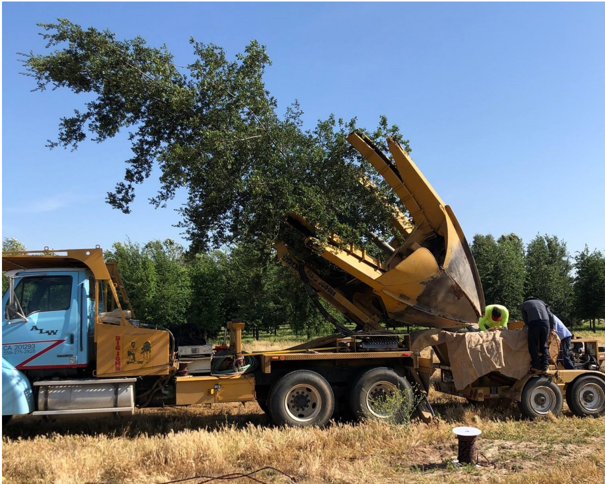
Hydraulic tree spade. Photo credit: Photo credit: Dane Jensen, West Coast Arborists
