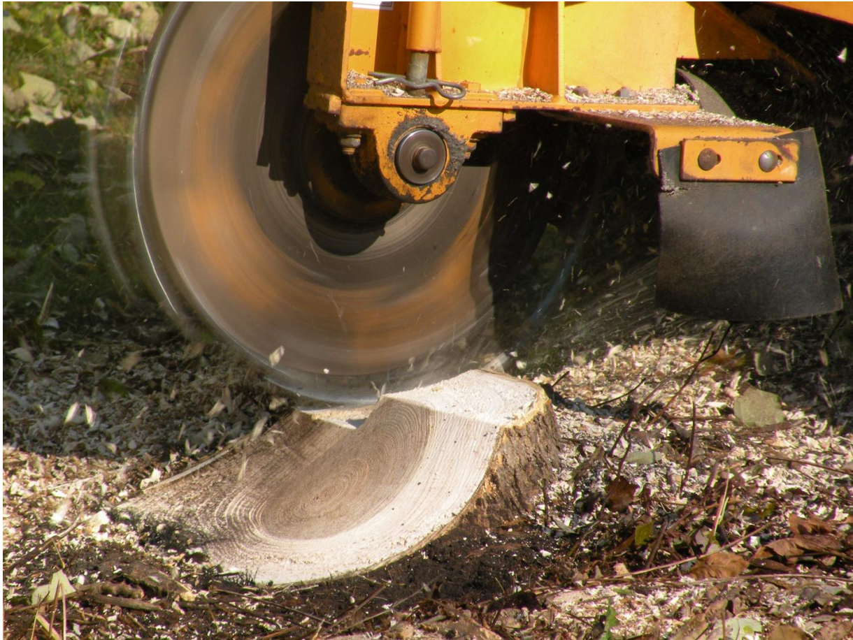
Grinding wheel in action and partially ground stump. http://www.stumpgrinding-mn.com/
