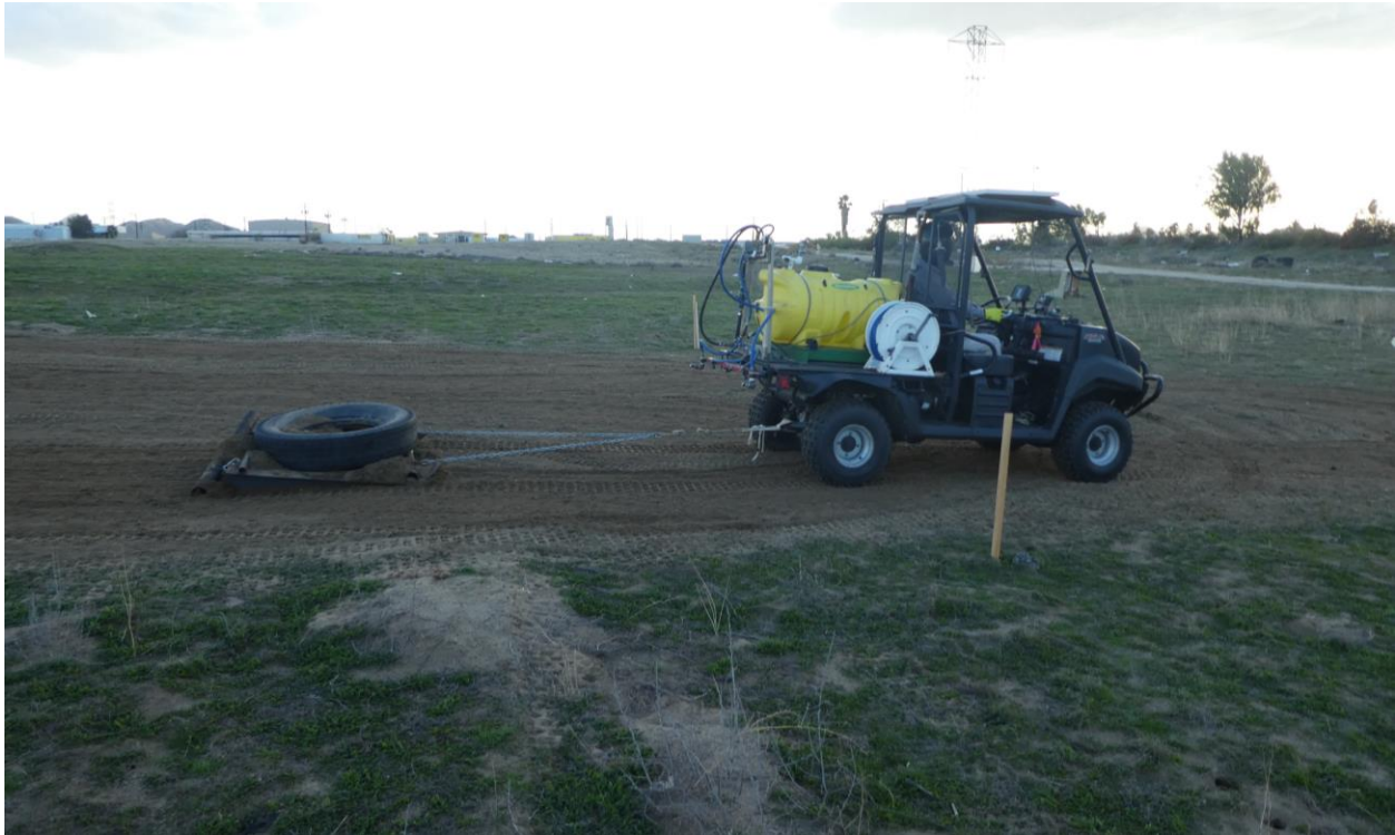
A 4x4 UTV pulling a modified harrow weighted down by an old tire as a winter seedbed treatment for a shrub restoration plot. Note that there is low residual plant cover and weeds are small. Photo credit: Ryan Lawler.
